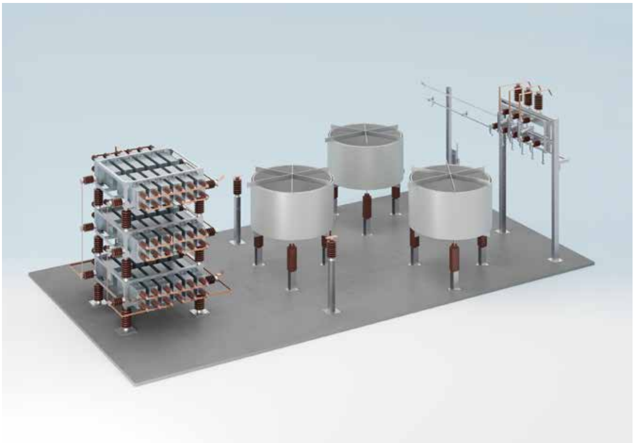
Fig. 43: PULSE shield: 3rd harmonic filter, 15 Mvar, 24 kV equipped with disconnector switch and phase CT, installation area: 12×8m
