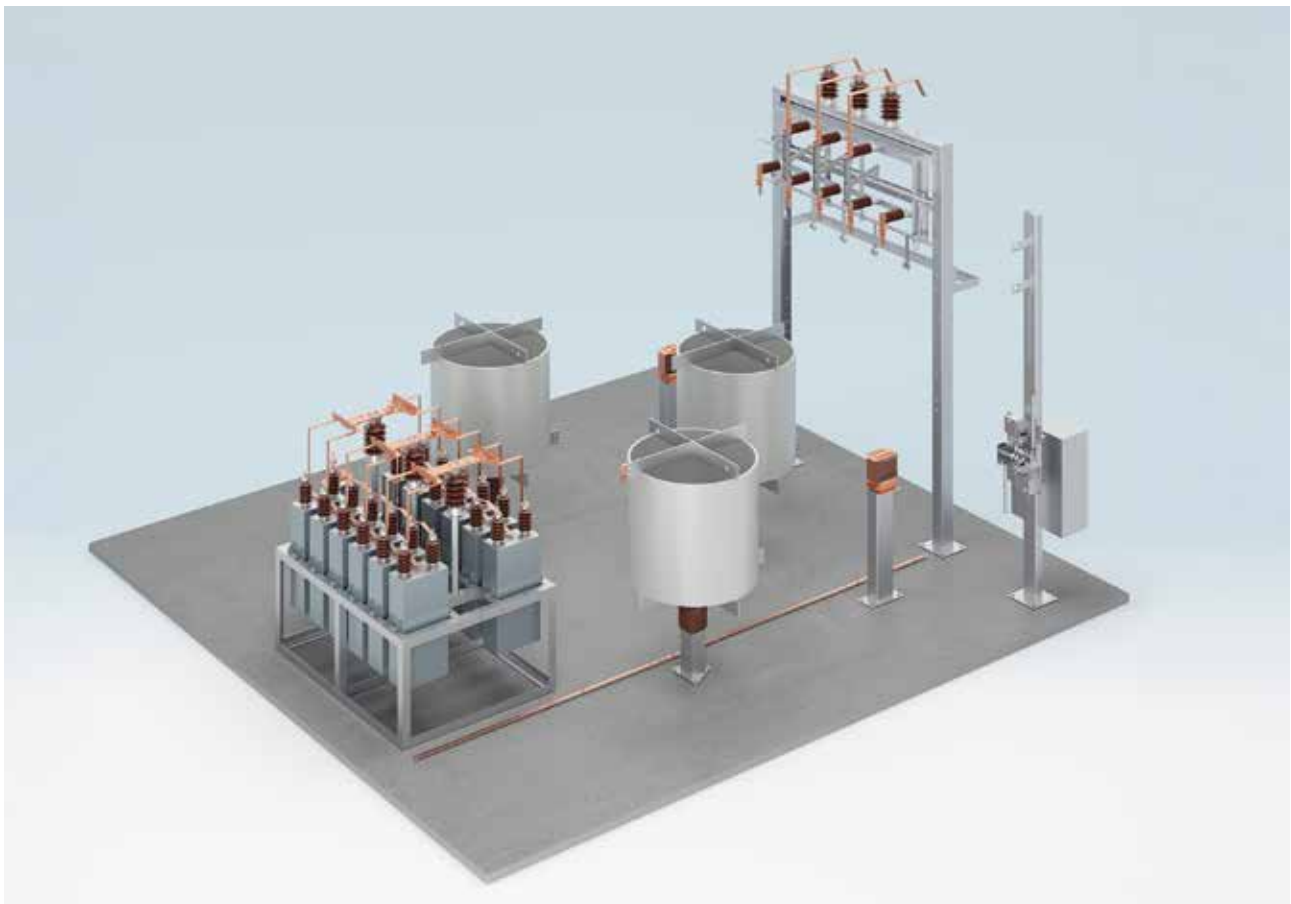
Fig. 41: PULSE shield: 5th harmonic filter, 3 Mvar, 12 kV equipped with disconnector switch and phase CT, installation area: 6.5×6.5m
