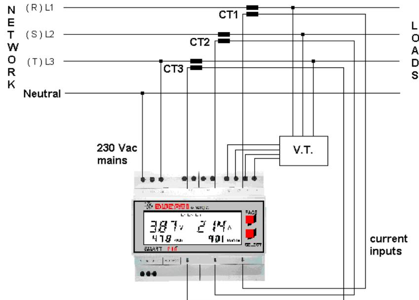
FIG 11 - CT and VT indirect three-phase connection
