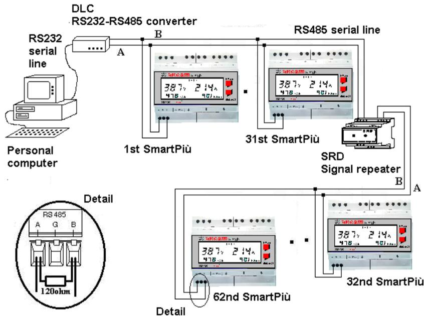
FIG 3 - Network with more than 31 analyzers
