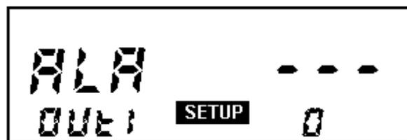
**FIG 43 - Setting of alarm on OUT1 output**
