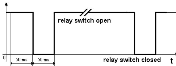
FIG 41 - Signal timing on the terminals of the OUT1 output
