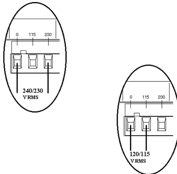
**FIG 9 - Power supply connections**
