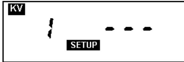
FIG 35 - Page for setting the VT transformation ratio
