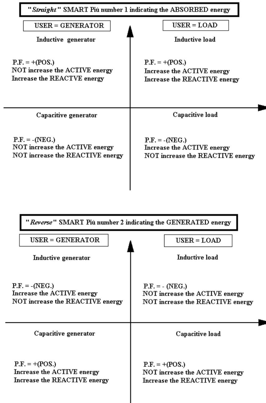
**FIG 16 - Pair of SMART Più for the measurement of the absorbed and generated energy**
