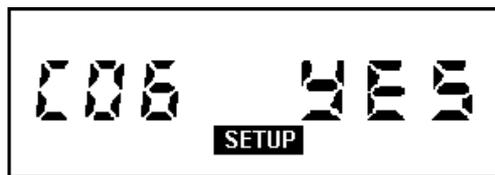
FIG 38 - Enabling the Cogeneration function
