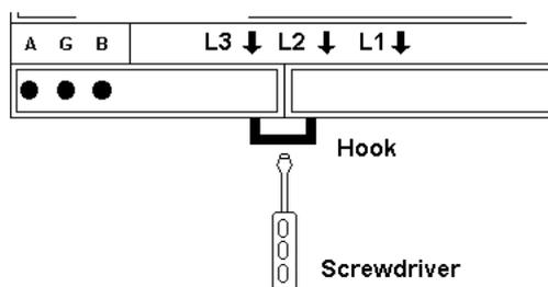
FIG 8 - DIN rail mount
