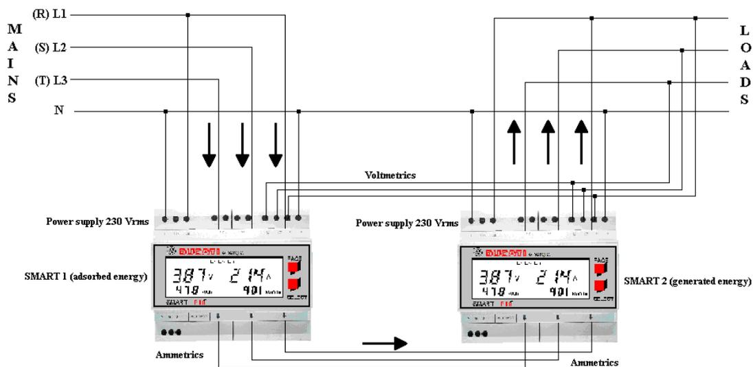
FIG 15 - Two SMART Più connected in opposition for the Cogeneration measurement
