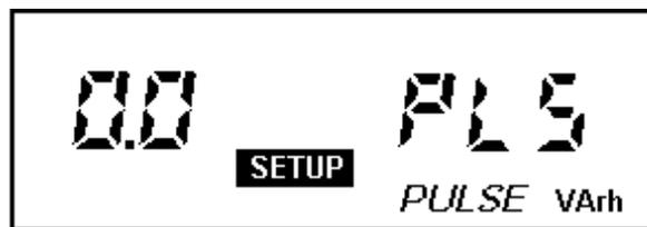
**FIG 42 - Pulsed output associated with the reactive energy (Varh/pulse)**
