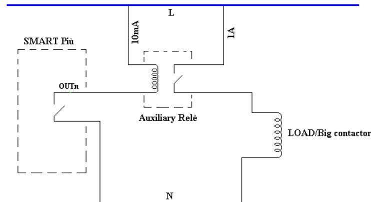
FIG 45 - Auxiliary relay for alarms outputs
