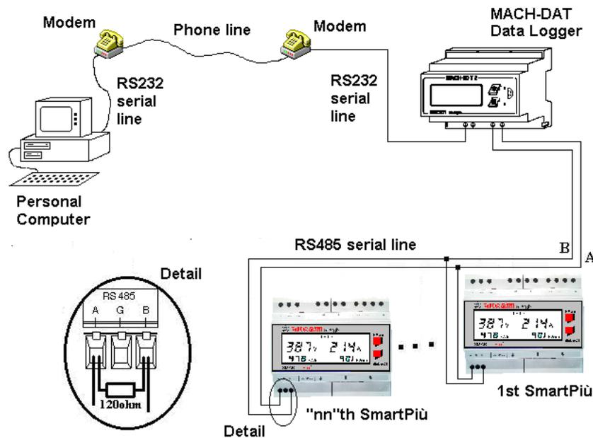
FIG 4 - Network with “DAT” data logger and modem
