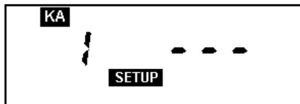
FIG 36 - Page for setting the CT transformation ratio
