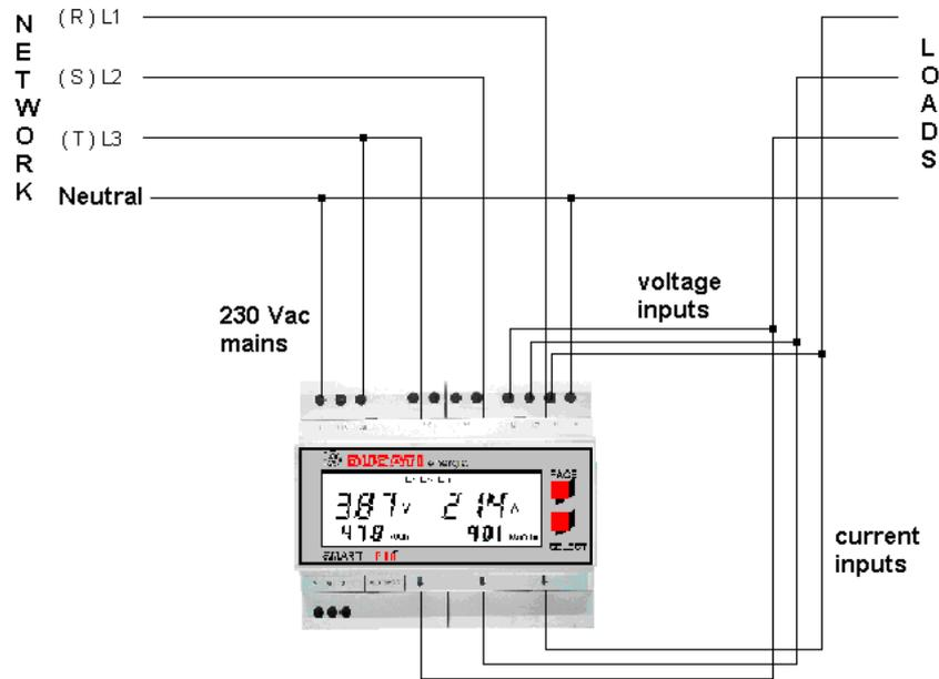
FIG 10 - Direct three-phase connection on the voltmeter and ammeter inputs
