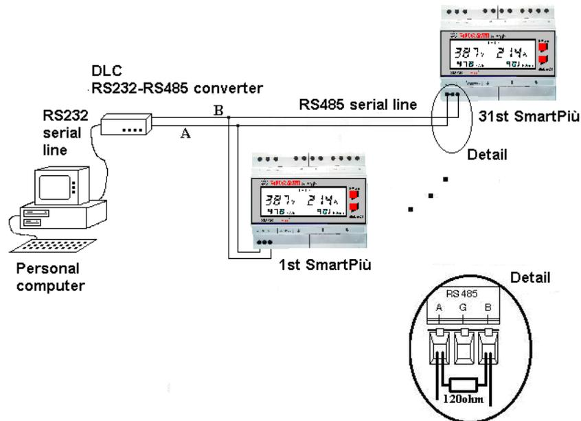
FIG 2 - Network with up to 31 analyzers
