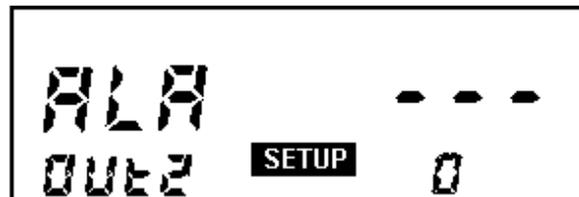
FIG 46 - Setting of alarm on OUT2 output
