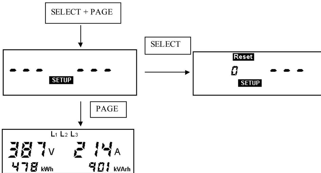
**FIG 6 - Press SELECT to enter the Setup menu**
