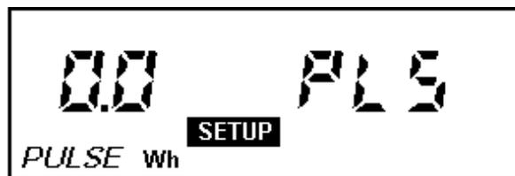
FIG 40 - Pulsed output associated with the active energy (Wh/pulse)
