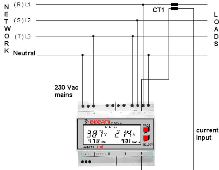
**FIG 14 - Balanced three-phase connection**
