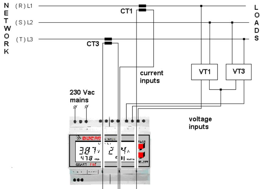
FIG 12 - Indirect three-phase connection with 2 CTs and 2 VTs
