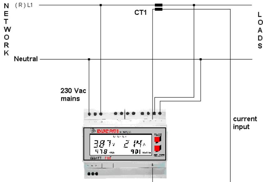
FIG 13 - Single-phase connection
