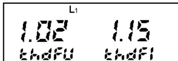
FIG 27 - Voltage's and current's ThdF – normal visualisation
