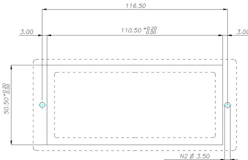
**FIG 60 - Frame for panel mount**
